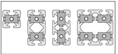
The standard connecting plates can be arranged to match the way in which the profiles are fitted.
