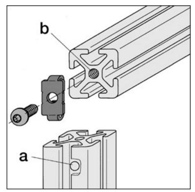
The necessary thread (b) is tapped directly into the core bore of the profile.
