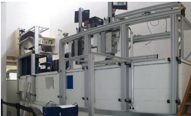
The calibration wall made of item profiles is perfectly adapted to its surroundings.
