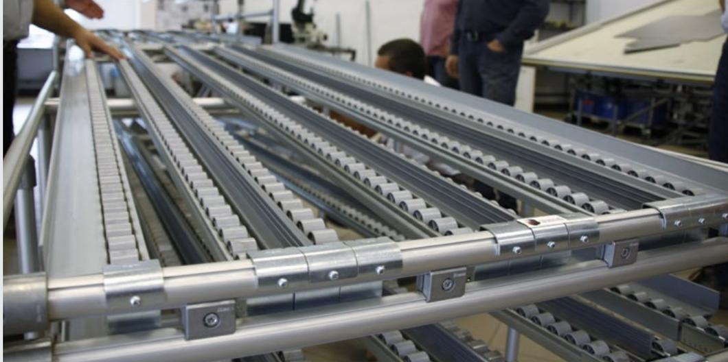
FIFO rack with roller conveyor in production
